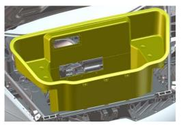
3. Haldex control unit fixing elements removal.
