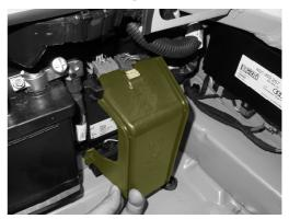
Install the cover on the Haldex control unit and check 5. the clip is correctly embedded.
